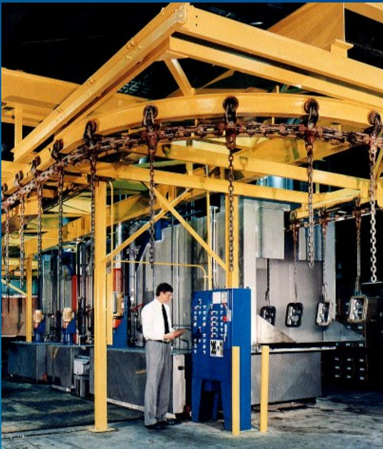
**STAINLESS STEEL WASHER** - Large parts are prepared for painting in a stainless steel washer with an overhead monorail conveyor system.
