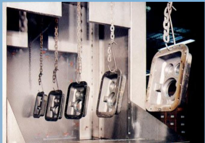
*PRECISION PARTS - Machined parts are cleaned and phosphated prior to assembly and painting.*
