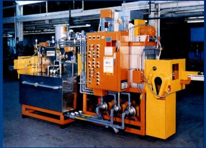
**AUTOMATIC IN-LINE PROCESSING** - Tooling fixtures are diverted to this 2-Stage combination washer/drier then returned to the production line.
