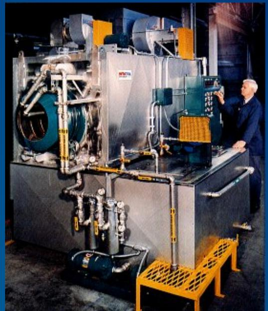
**AUTOMOTIVE** - Combination 2-Stage drum washer with integral dry-off section for processing small parts.
