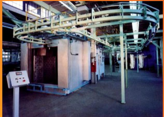
**SPECIALIZED CONVEYOR OVENS** - Gas or electric ovens with special conveyors including loaders/unloaders and cooler for electronic parts, air bag housings, plastic parts and special castings.
