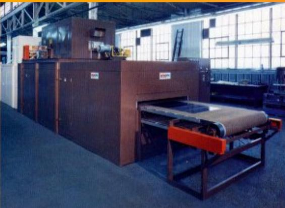
**SILK SCREEN** - Electric radiant and electric convection oven with cooler to process metal, vinyl and fabric silk screened substrates.
