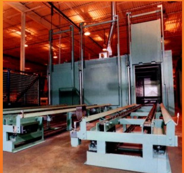
**PLASTICS** - Molded plastic parts are preheated in this oven and conveyor prior to test and further processing.
