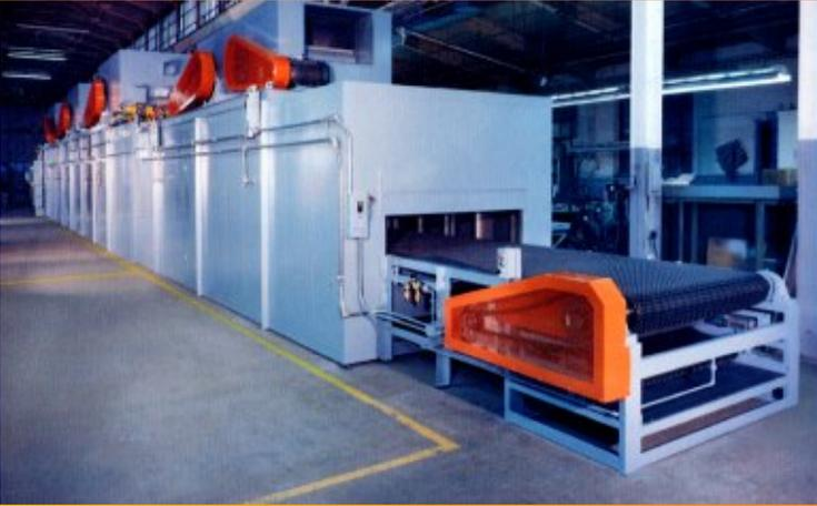
**FOUNDRY** - Multi-zone conveyorized convection oven and cooler for curing water-based coating on sand cores.
