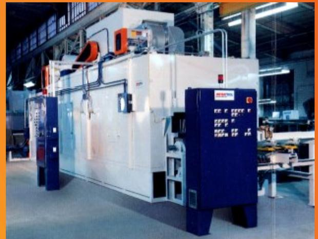
**WOOD PRODUCTS** - Gas-fired, high velocity convection oven for curing water borne coatings on exterior wood siding. Cure time: 6 seconds at speeds of 400 fpm.
