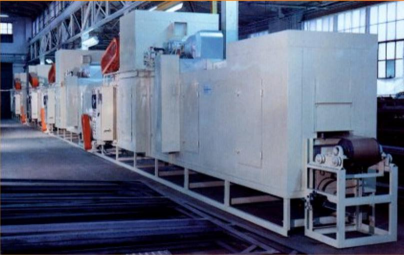
**RUBBER** - Multi-zone convection oven for curing rubber extrusions in seconds at speeds of 60 fpm.
